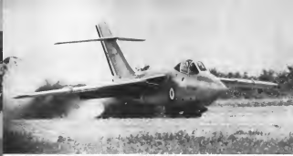
LANDING BARBUDIUS generates a cloud of dust as retractable landing gear hits the ground in testing. The aircraft, which was built instead of conventional gear, also utilizes a drag chute for deceleration.
